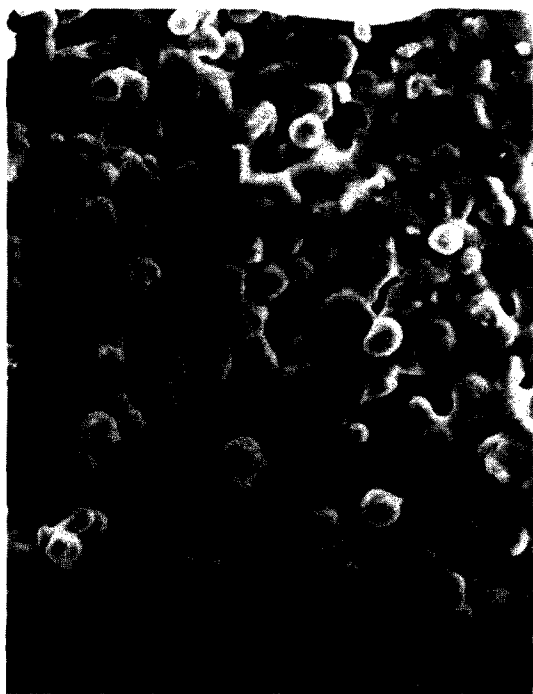
Figure 5 Scanning electron micrograph of 60/40 starch/EPMA blend made at 100 rev min -1 mixer speed and 10 min mixing time
